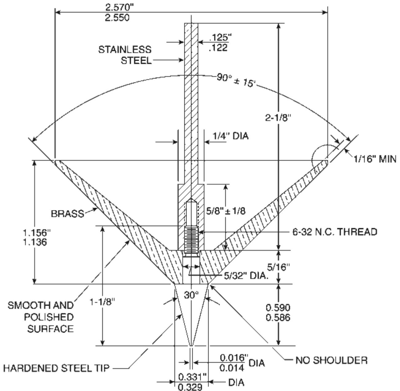
Figure 2. Penetration cone dimensions. DIA, diameter; N.C., National Coarse.
