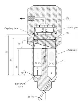
Figure 2. Flow-through cell designed for lipid-filled soft gelatin capsules (dimensions in mm).
